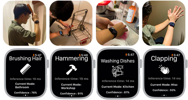
Figure 2: Our WatchHAR system running in real-time on an Apple Watch Series 7 (45mm), demonstrating activity recognition across four different contexts: brushing hair, hammering, washing dishes, and clapping.
